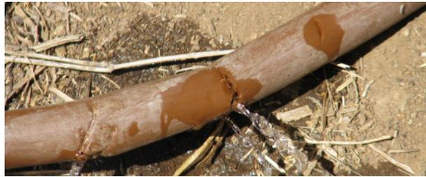
Figure 4. Damage to an irrigation water pipeline [25]
