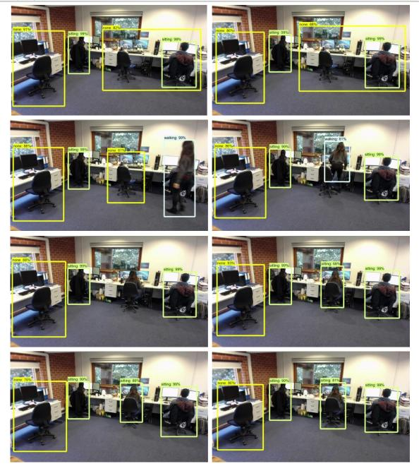
Figure 9. Example snapshots at various times of the day of the experimental test of the detection and recognition of occupants within an office space using the deep learning occupancy activity detection approach
