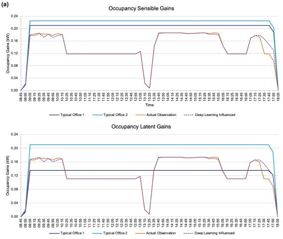
Figure 15. Occupancy heat gains within the office space during the detection period of 09:00 - 18:00: sensible heat gains (a); latent heat gains (b)
