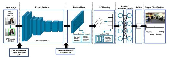
Figure 2. Convolutional Neural Network (CNN) based deep learning model configured for the training of the model for occupancy activity detection and recognition
