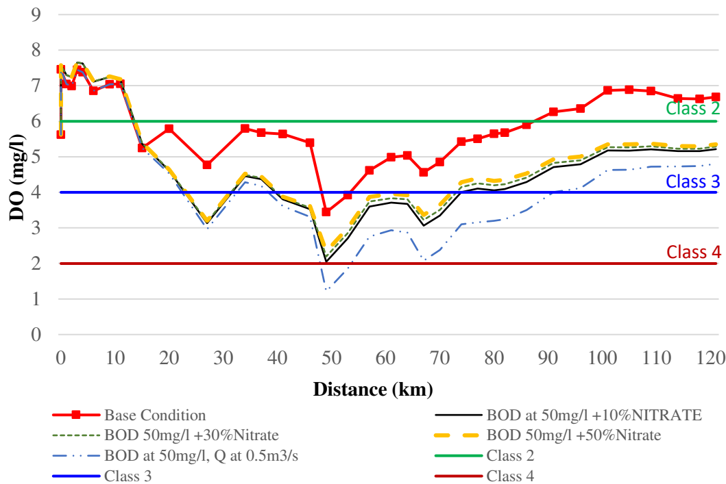
Figure 7. DO concentrations along with the downstream of Lam Takhong River with different BOD 5 concentrations for point sources and nutrient augmentation.
