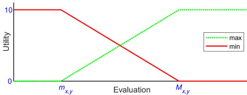
Figure 1. Utility function for maximization and minimization criteria
