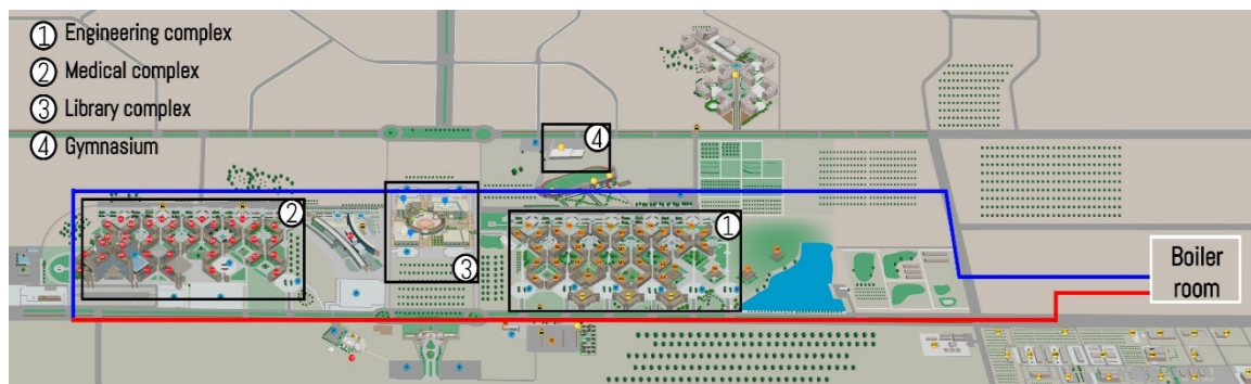
Figure 2. A simplified schematic diagram of the existing DH network at JUST.
