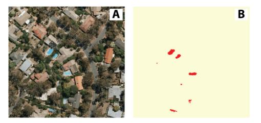
Figure 2. Sample  $640 \times 640$  pixel satellite image (Panel A) and SVM identified swimming pools (Panel B)
