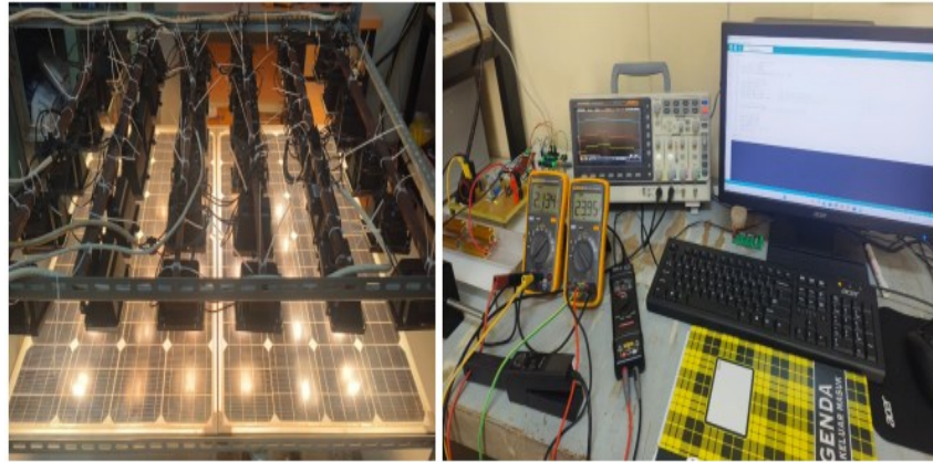
Figure 4. Experimental hardware (solar simulator, converter, and measurement equipment)
