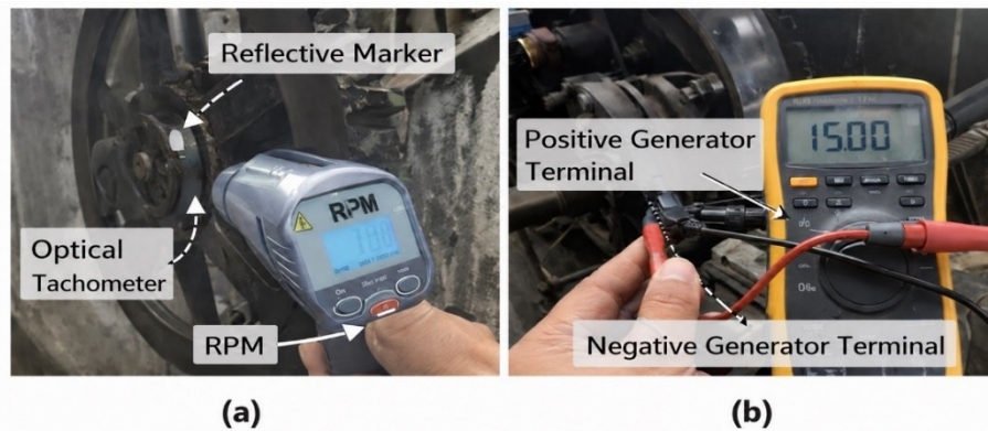
Figure 4. Measurement arrangements used in the two post-installation operational runs.
