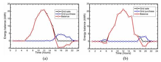
Figure 12. Hourly energy balance in the grid: HOMER results (a) and SAM results (b)
