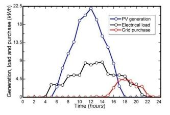
Figure 8. HOMER results of the PV generation, electrical load and grid purchase
