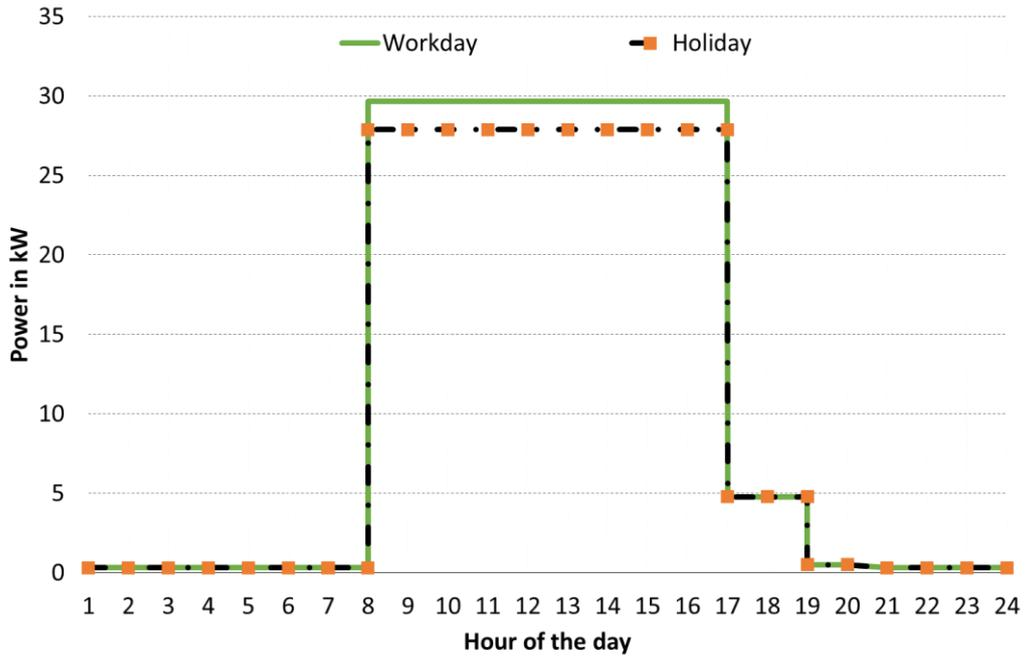
Figure 5. Accumulated daily electrical demand profile during workdays and holidays considering 100 km as daily distance covered by e-bikes
