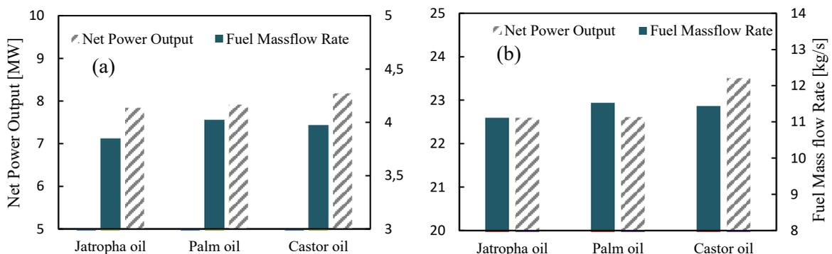
Figure 4. Net power output and fuel mass flow rate of additional gas turbine unit using three biofuels for: (a) booster heater replacement; (b) HTF heater replacement
