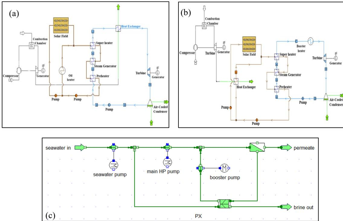
Figure 3. Schematic of proposed systems: replacement of booster heater with GT (a); replacement of HTF heater (b); RO plant equipped with an energy recovery system (c)
