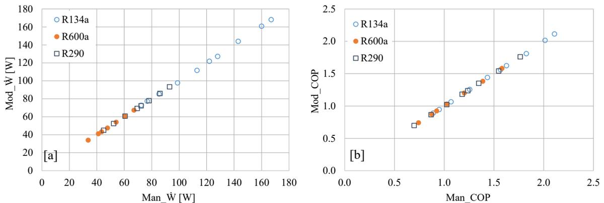
Figure 3. Simulation model data vs manufacturer data for [a] compressor energy consumption and [b] refrigerator COP
