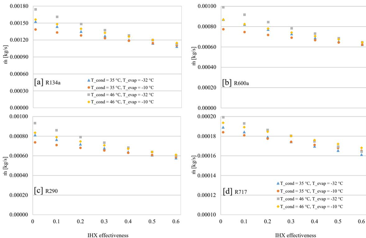
Figure 7. Refrigerant mass flow ( $\dot{m}$ ) vs IHX effectiveness,  $T_{cond}$ , and  $T_{evap}$ , for: [a] R134a, [b] R600a, [c] R290, and [d] R717
