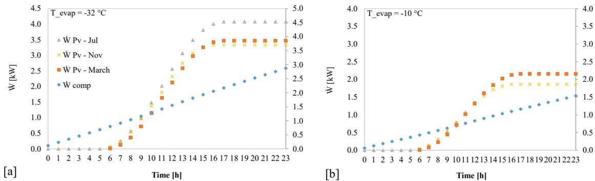
Figure 13. Cumulative PV power production and compressor energy consumption for the R290 refrigeration system at an evaporation temperature of [a]  $-32\text{ }^{\circ}\text{C}$  and [b]  $-10\text{ }^{\circ}\text{C}$
