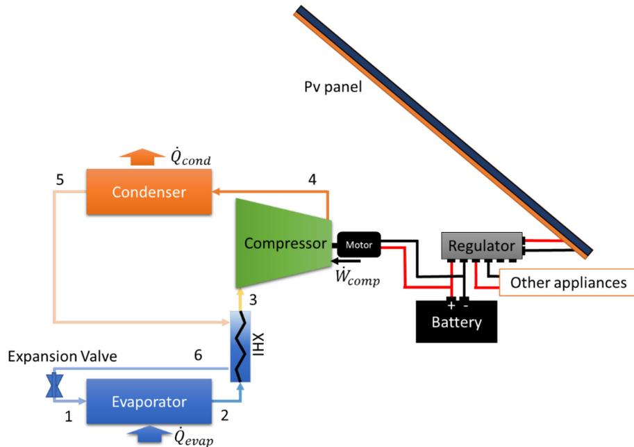
Figure 1. Scheme of the horizontal solar vapour compression refrigerator with internal heat exchanger
