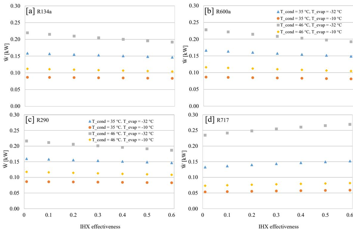
Figure 6. Compressor power consumption ( $\dot{W}$ ) vs IHX effectiveness,  $T_{cond}$ , and  $T_{evap}$ , for: [a] R134a, [b] R600a, [c] R290, and [d] R717
