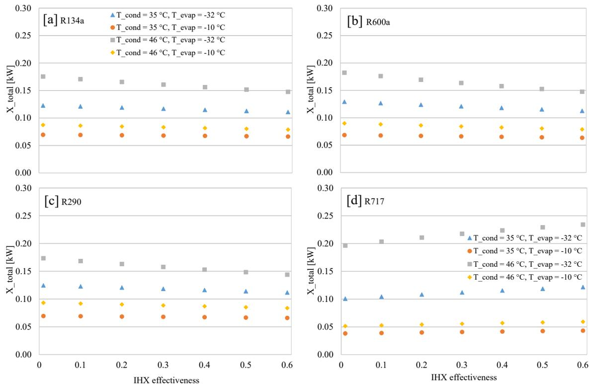
Figure 10. Total exergy destruction vs IHX effectiveness,  $T_{cond}$ , and  $T_{evap}$  for: [a] R134a, [b] R600a, [c] R290, and [d] R717.
