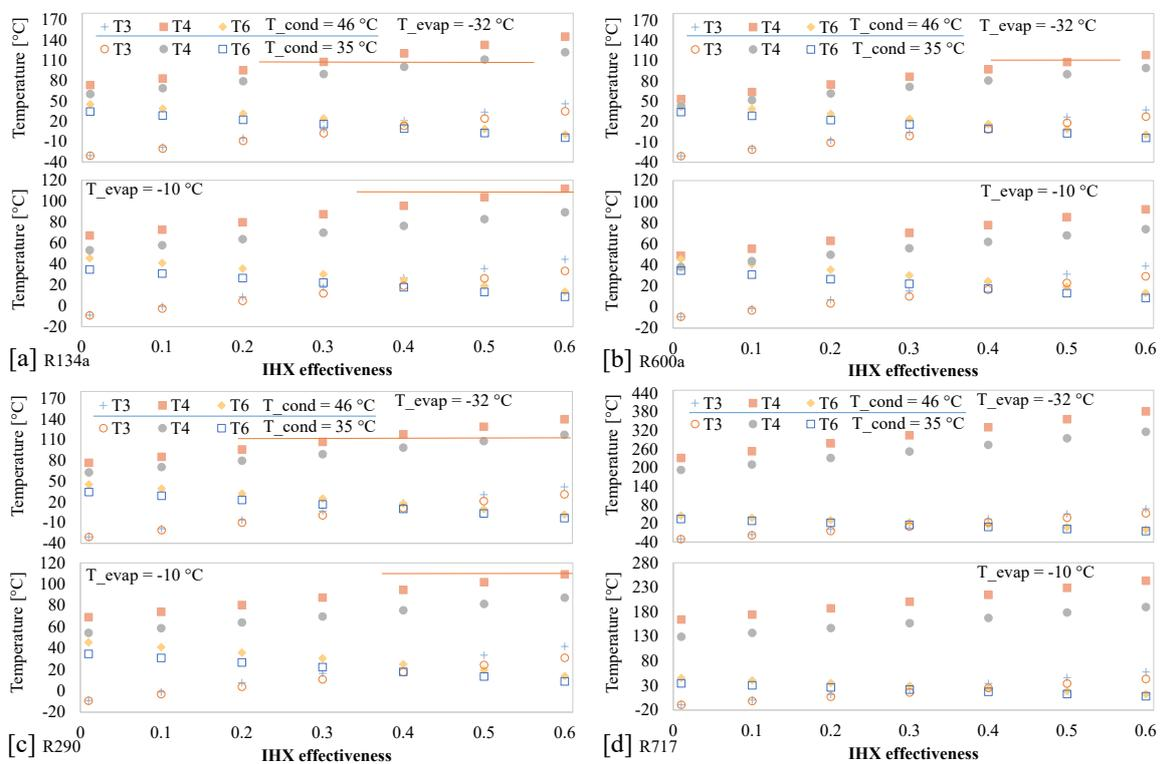
Figure 8. Temperatures at the outlet of the compressor and IHX vs IHX effectiveness,  $T_{cond}$ , and  $T_{evap}$ , for: [a] R134a, [b] R600a, [c] R290, and [d] R717
