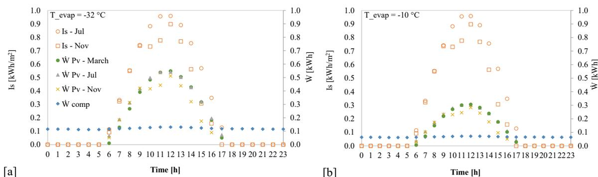
Figure 12. Solar irradiation ( $I_s$ ) vs PV power production ( $\dot{W}_{Pv}$ ) and compressor energy consumption ( $\dot{W}_{comp}$ ) for the R290 refrigeration system at an evaporation temperature of [a] -32 °C and [b] -10 °C
