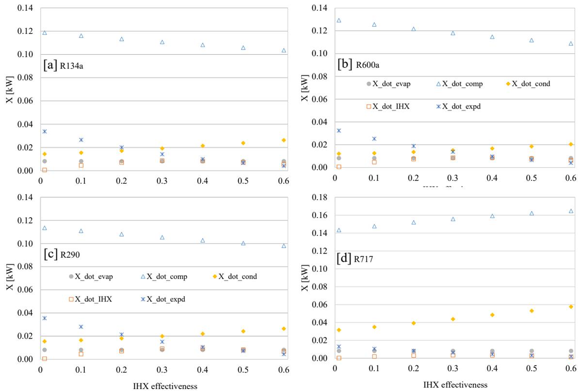
Figure 11. Exergy destruction in each component vs IHX effectiveness for: [a] R134a, [b] R600a, [c] R290, and [d] R717
