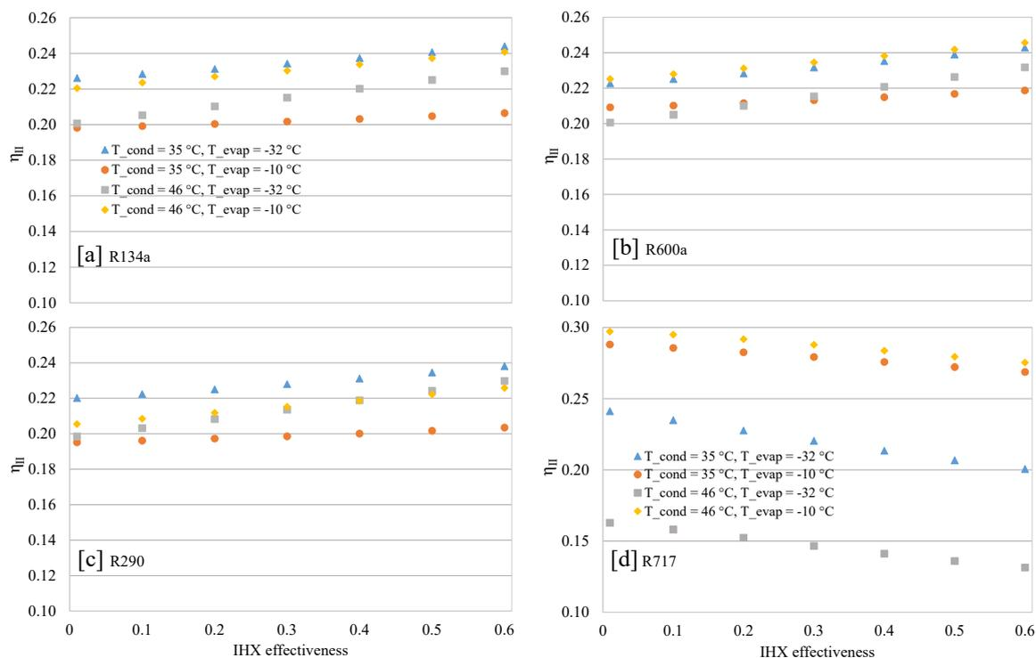
Figure 9. 2<sup>nd</sup> law efficiency vs IHX effectiveness,  $T_{cond}$ , and  $T_{evap}$  for: [a] R134a, [b] R600a, [c] R290, and [d] R717
