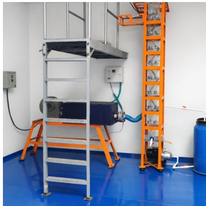
Figure 2. Laboratory cooling tower system with perforated inclined plates and associated equipment
