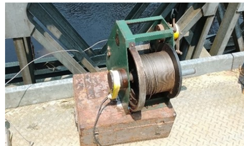
Figure 6. Manual winch used during measurements
