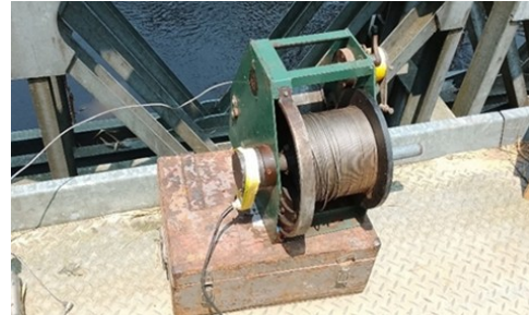
Figure 5. Manual winch used during measurements.
