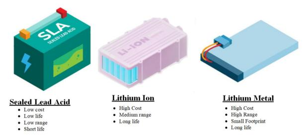
Figure 5. Types of EV batteries
