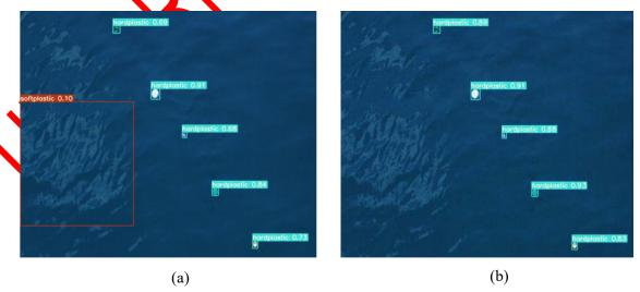
Figure 7. Detection results in the presence of surface reflection artifacts: (a) results obtained with the standard YOLOv7 model and (b) results obtained with the proposed method.
