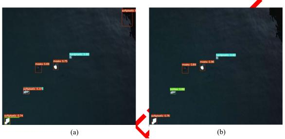
Figure 8. Detection performance on small and low-contrast floating debris: (a) results obtained with the standard YOLOv7 model and (b) results obtained with the proposed method.
