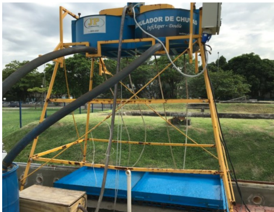
Figure 10. Simulator and the collector plates [52]
