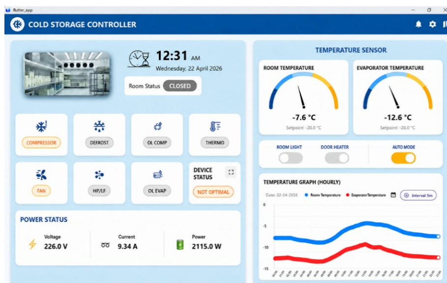
Figure 3. Monitoring interface of the smart cold storage controller showing thermal condition, operating status, and electrical power parameters
