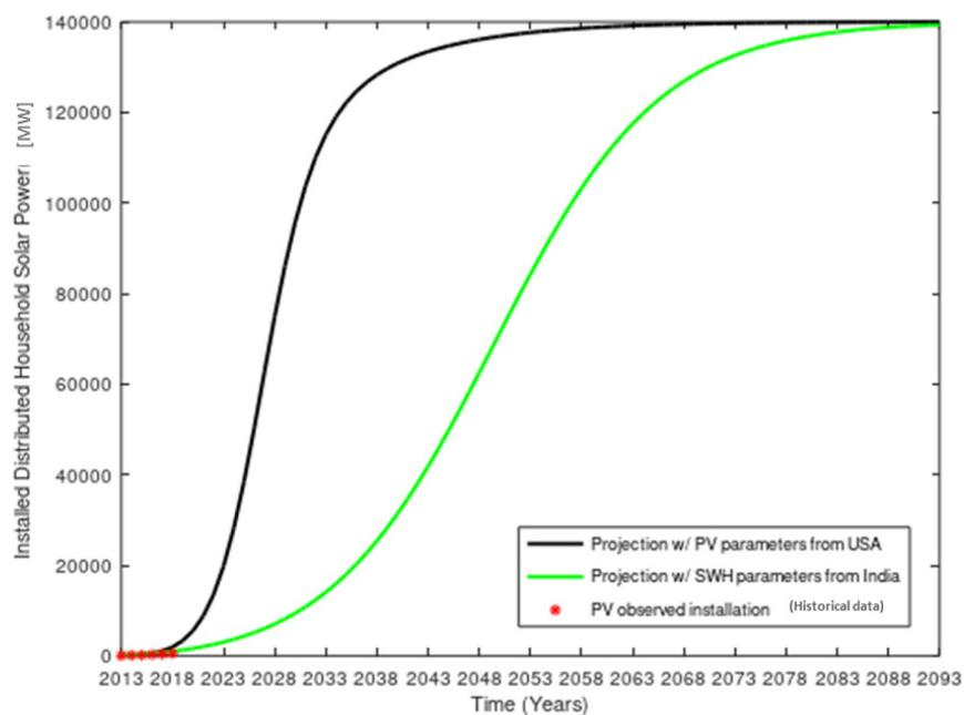
Figure 4. Projection of the rooftop PV market evolution in India using parameters from PV data from USA and from SWH data
