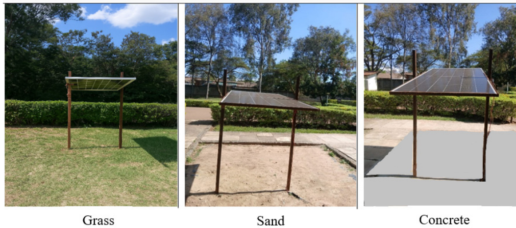
Figure 2. Image of the bifacial panel mounted on different surfaces
