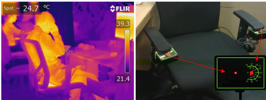
Figure 5. Thermal image of the thermal chair during the field test (a) and on board controls for seat and backrest heating (b)
