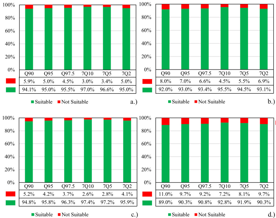
Figure 5. Weighted velocity usable area percentage for a.) Cyprinus carpio , b.) Hampala macrolepidota , c.) Oreochromis niloticus , d.) Hemibagrus nemurus
