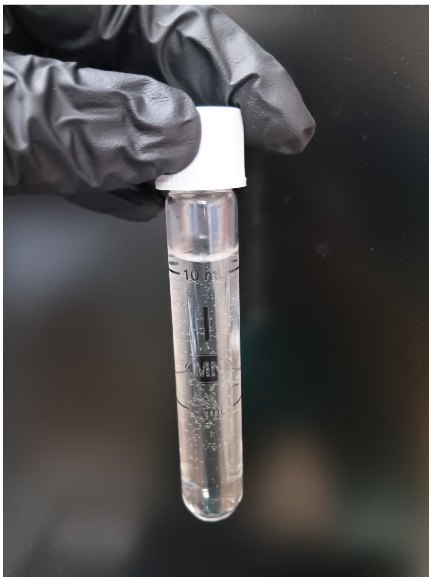
Figure 3. Air bubbles formed on the wall of glass cuvette
