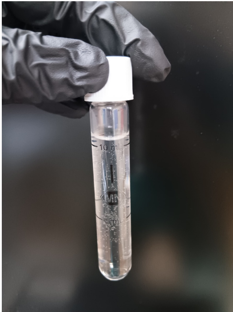
Figure 3. Air bubbles formed on the wall of the glass cuvette
