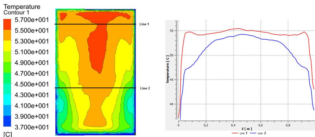
Figure 3. Temperature distribution on the upper surface of the PV panel from the numerical simulation
