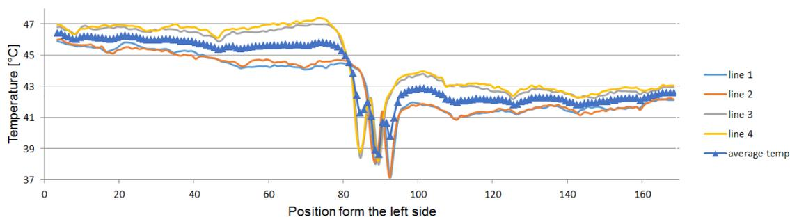
Figure 9. Temperature distribution on loaded and non-loaded panel
