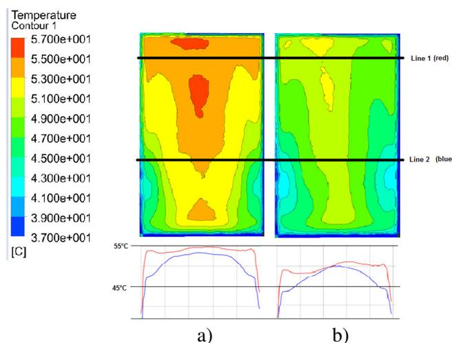
Figure 5. Temperature distribution on the upper surface of the PV panel from the numerical simulation for two different heat loads of PV panel: 488 W/m<sup>2</sup> (a) and 416 W/m<sup>2</sup> (b)
