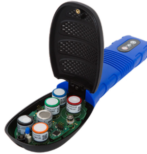
Figure 5. GrayWolf DirectSense II smart probes [38]
