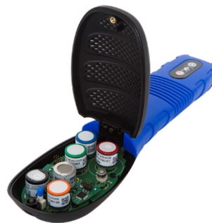
Figure 5. GrayWolf DirectSense II smart probes [38]
