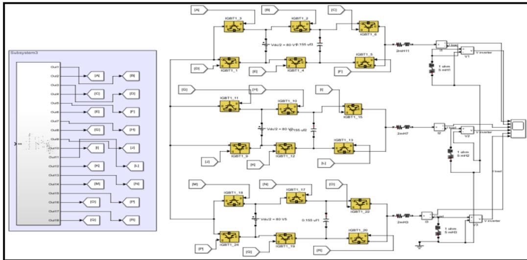
Figure 3. Three phase seven-level packed U-Cell Inverter
