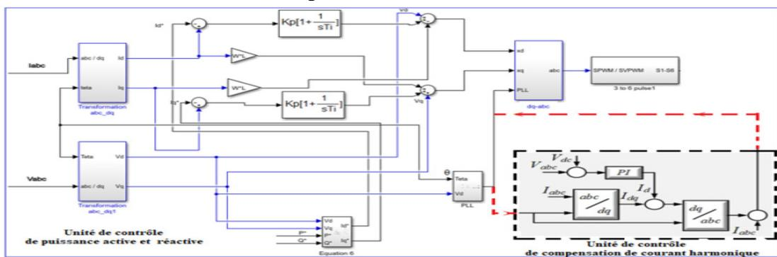
Figure 5. Current harmonic control and compensation unit
