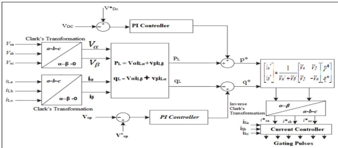
Figure 6. Block diagram of IRP based control algorithm
