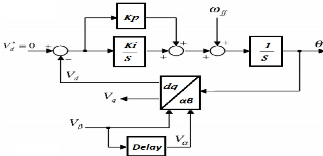
Figure 7. Phase locked loop algorithm
