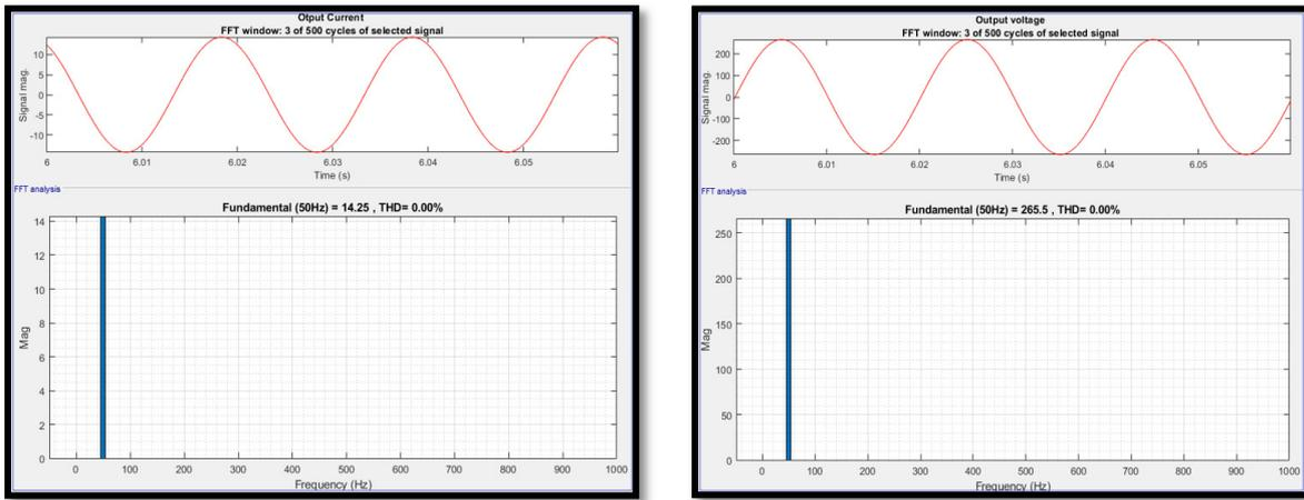
Figure 13. FFT spectrum current and voltage by the SVPWM control
