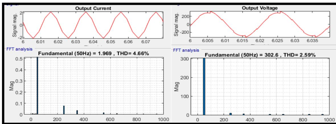
Figure 10. Grid current and voltage FFT spectrums before filtering
