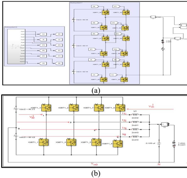
Figure 2. (a) Seven-level CHB inverter (one phase);
