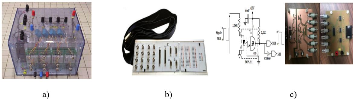
Figure 14. a) Three-phase voltage inverter; b) CLP1104DSP; c) electronic galvanic isolation board
