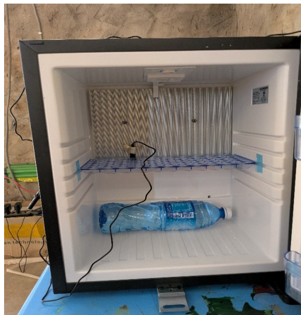
Figure 4. Cabinet space of the vapour absorption refrigerator with bottled water
