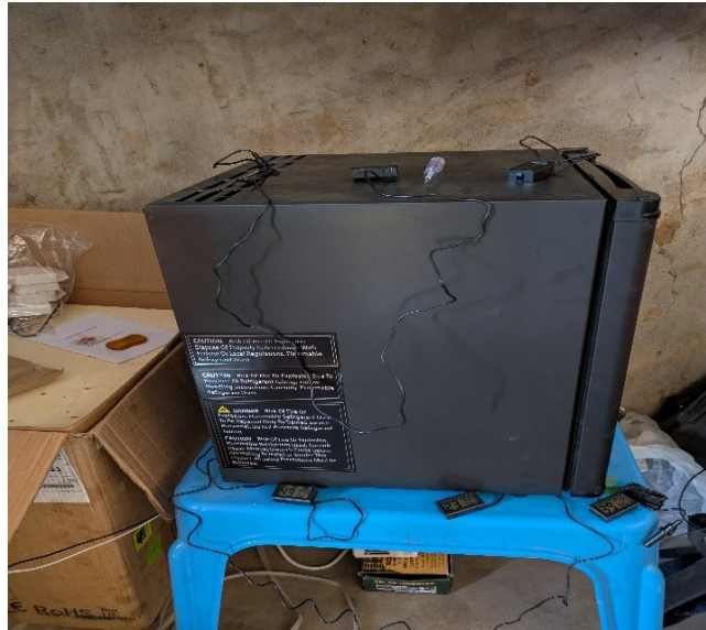
Figure 3. Experimental setup of the vapor absorption refrigerator during load testing
