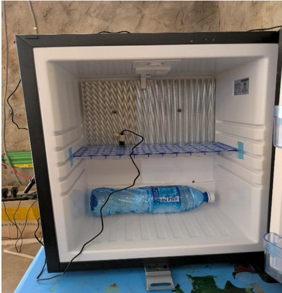
Figure 4. Cabinet space of the vapor absorption refrigerator with bottled water
