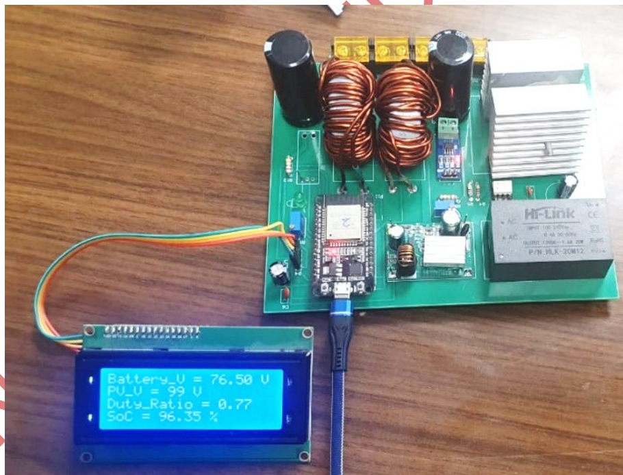
Figure 15, The voltage and state of charge for golf cart powered by pv panels.
